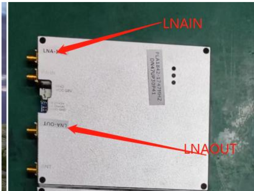
LNAIN is the upstream input, LNAOUT is the upstream output Upstream signal input is about -40dbm
