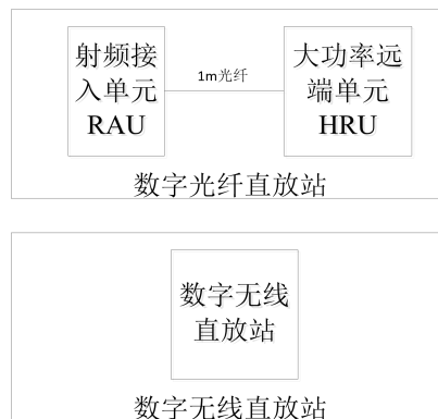
图1 The shortest link digital repeater single-item RF index test block diagram
